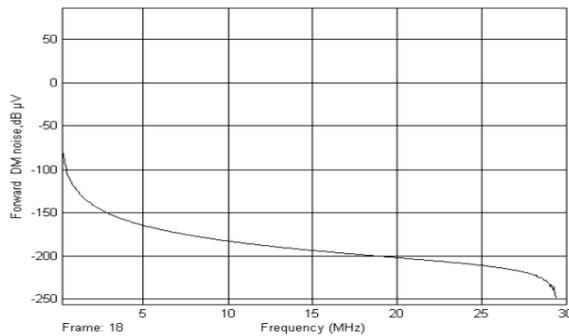
Figure 2 DM noise generated by a simulated Forward Converter with 47  $\mu\text{F}$  bulk filter capacitor
