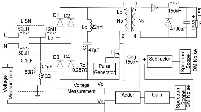
Figure 1(a) Block diagram of a Forward converter and noise measurement set-up including LISN
