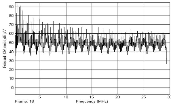
Figure 6 CM noise generated by simulated Forward Converter with 150pF MOSFET drain to earth capacitance
