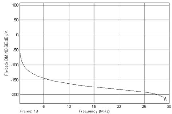
Figure 7 DM noise generated by a simulated Fly-back Converter with 47 μF bulk filter capacitor
