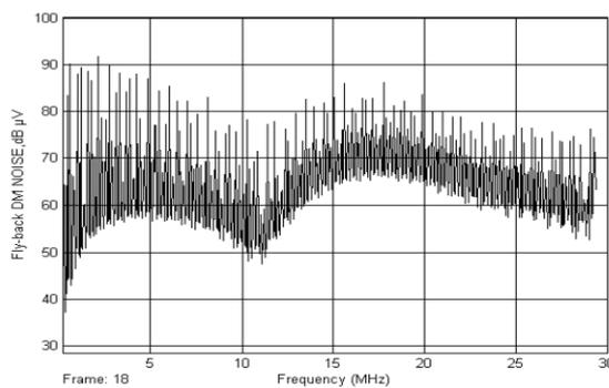
Figure 10 DM noise generated by a simulated Fly-back converter having a Bulk Filter capacitor of 47 μF with 22 nH ESL, 0.287 Ω ESR, a 12nH path inductance and a 150pF capacitor added representing the stray capacitor between MOSFET switch drain and earth terminal
