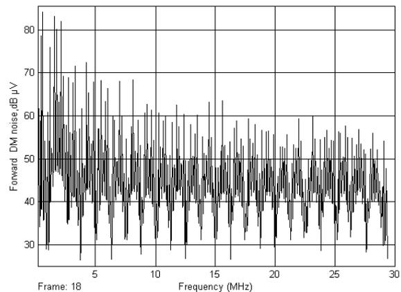
Figure 5 DM noise generated by a simulated Forward Converter with 47  $\mu\text{F}$  bulk filter capacitor with 0.287  $\Omega$  ESR and 22nH ESL, 12 nH path inductance and 150pF MOSFET drain to earth capacitance
