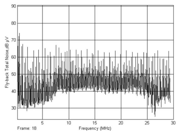
Figure 17 Total Noise generated by a simulated Fly-back converter with a 150pF capacitor added between MOSFET switch drain and earth terminal
