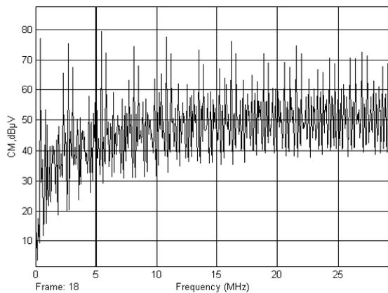
Figure 16 CM noise generated by a simulated Soft Switching Fly-back converter with a 150pF capacitor added between MOSFET switch drain and earth terminal
