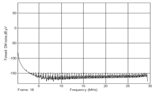
Figure 3 DM noise generated by a simulated Forward Converter with 47  $\mu\text{F}$  bulk filter capacitor with 0.287  $\Omega$  ESR and 22nH ESL
