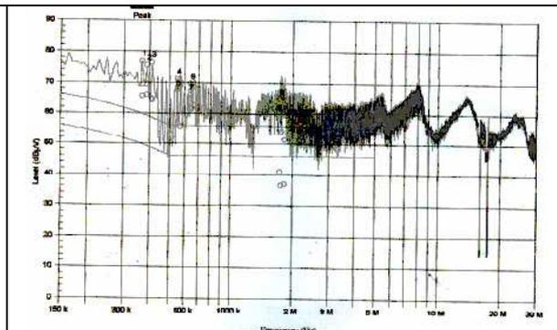
Figure 19 Conducted Emission Measurement of Fly-back Converter Prototype
