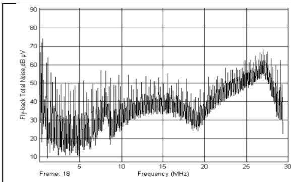
Figure 18 Total Noise generated by a simulated Fly-back converter with a 150pF capacitor between MOSFET switch drain and earth terminal and a 2.2 nF inter-winding capacitance added between 1 & 4 terminals (refer Figure 1) of the transformer
