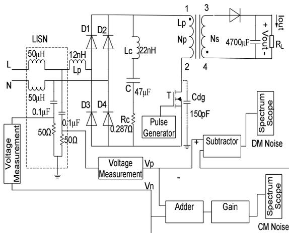
Figure 1(b) Block diagram of a Fly-back converter and noise measurement set-up including LISN
