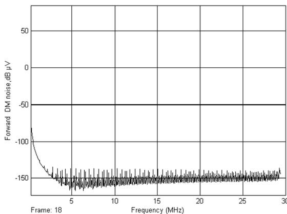
Figure 4 DM noise generated by a simulated Forward Converter with 47  $\mu\text{F}$  bulk filter capacitor with 0.287  $\Omega$  ESR and 22nH ESL and 12 nH path inductance
