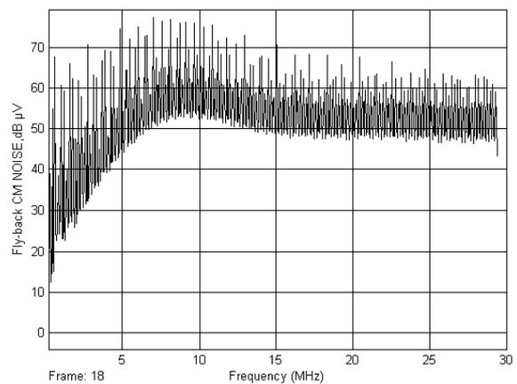
Figure 11 CM noise generated by a simulated Fly-back converter with a 150pF capacitor added between MOSFET switch drain and earth terminal
