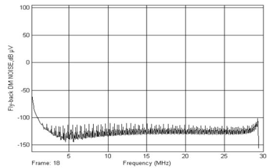
Figure 9 DM noise generated by a simulated Fly-back converter having a Bulk Filter capacitor of 47 μF with 22 nH ESL and 0.287 Ω ESR and a 12nH path inductance
