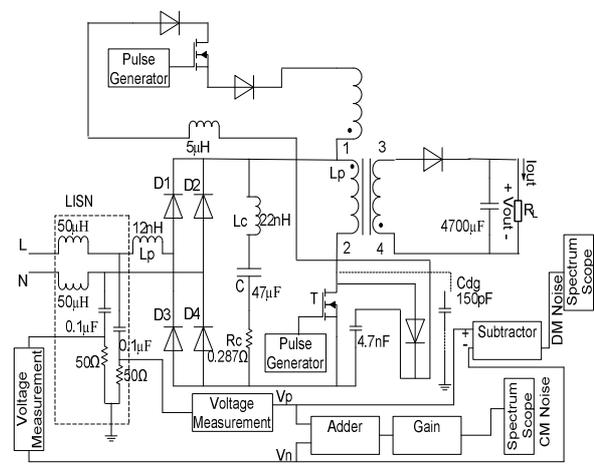
Figure 1(c) Block diagram of a ZVT Fly-back converter and noise measurement set-up including LISN
