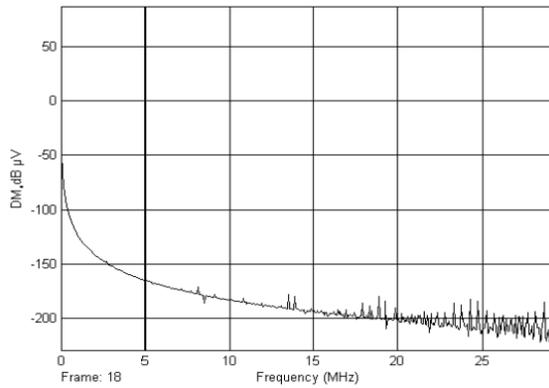
Figure 14 DM noise generated by a simulated Soft Switching Fly-back Converter having 47  $\mu$ F bulk filter capacitor with 0.287 ESR, 22nH ESL and 12nH path inductance
