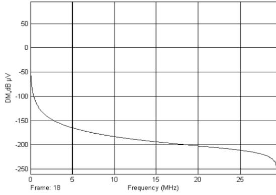
Figure 12 DM noise generated by a simulated Soft Switching Fly-back converter with a 47 $\mu$ F Bulk Filter Capacitor
