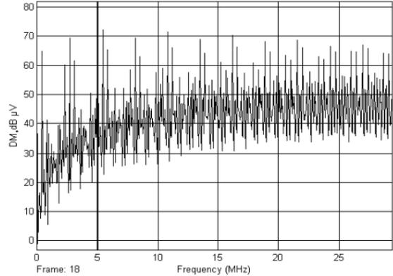
Figure 15 DM noise generated by a simulated Soft Switching Fly-back Converter having 47  $\mu$ F bulk filter capacitor with 0.287 ESR, 22nH ESL, 12nH path inductance and 150pF MOSFET drain to earth capacitance
