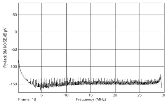
Figure 8 DM noise generated by a simulated Fly-back Converter having 47 μF bulk filter capacitor with 0.287 Ω ESR and 22nH ESL
