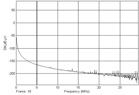
Figure 13 DM noise generated by a simulated Soft Switching Fly-back Converter having 47  $\mu$ F bulk filter capacitor with 0.287 ESR and 22nH ESL
